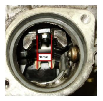
02Q casing – especialy Mk5 casings hase more material around bearings and are better for high torque engines.
