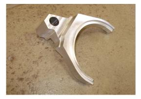
4 – Very often is possible by hard shifting demage (open) shifting elements on forks 1°-2° and 3°-4°, must be checked after every race/event and if is gap on fork bigger than 15,20mm must be element replaced, **standard gap is 14,95-15,00 mm** – see pics.
