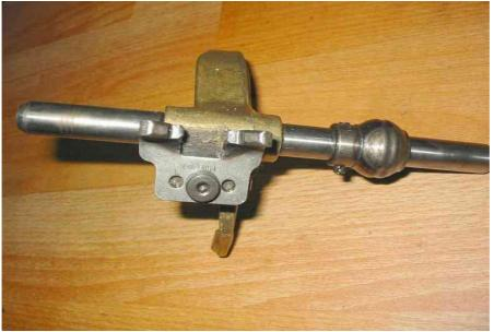
Replace complete fork 3°-4° by delivered Alu, secure by double pins !
