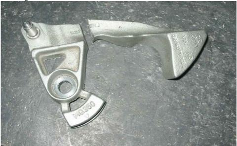
Replace the rivet in fork 1°-2° by delivered bolt, secure the nut by LOCTITE ! Hole in fork must be redriled to 8mm !
