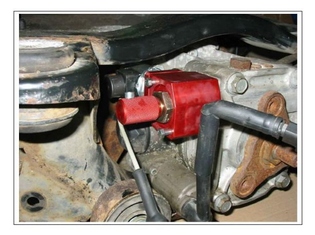
Install MHR(B) to this position enstead of original Haldex ECU. Use original seal and be careuful to right postion (bad position of sealing can close hydraulic chanels and couse bad function of system).
